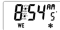
Fig. 3. Hot Water Only Mode, (Central Heating will switch on if room temperature falls below 5°C.)
